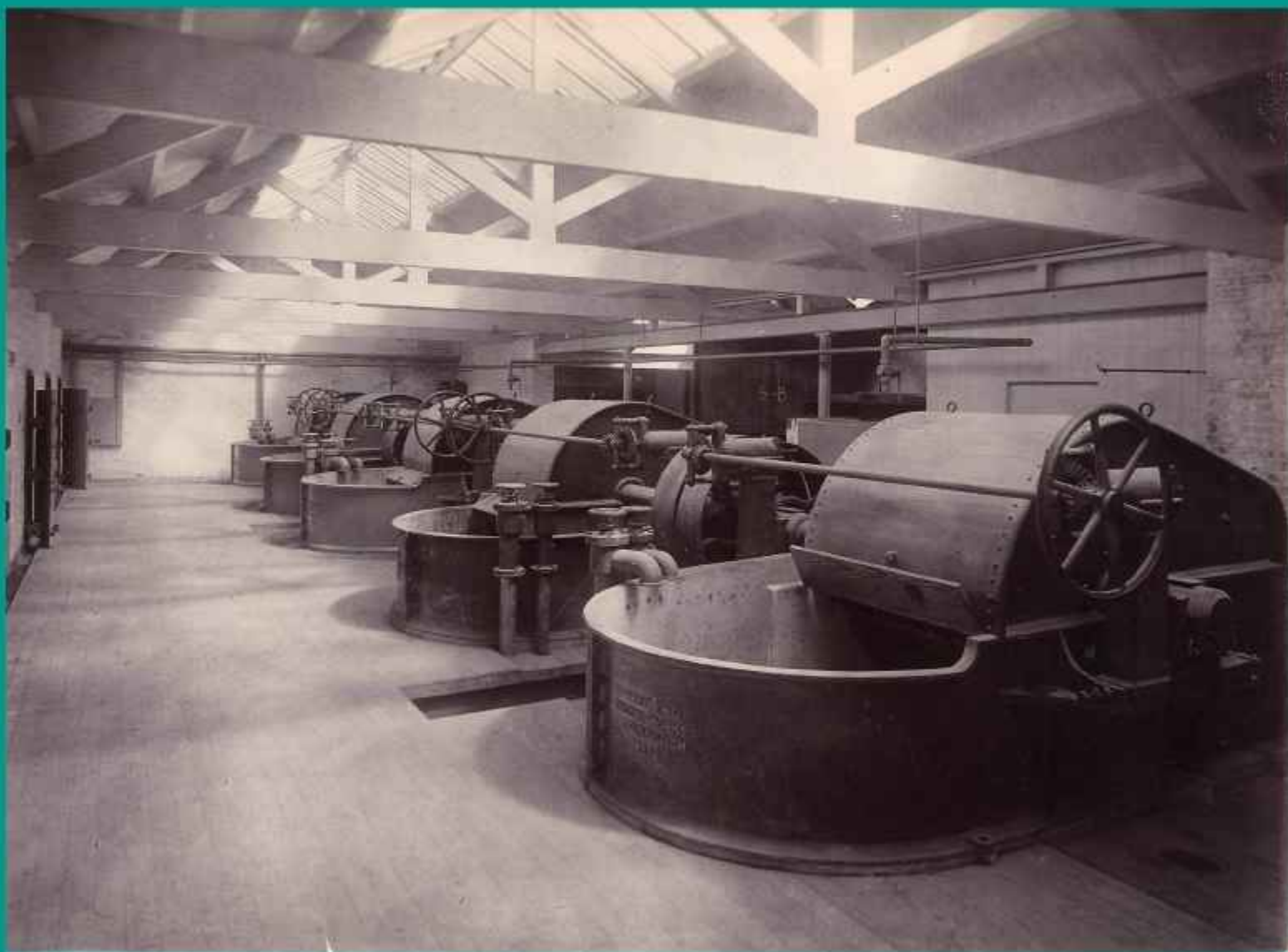
Five 'hollander' beaters were driven by the steam engine
